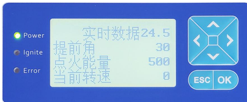
Indicator status and display of no camshaft sensor signal
